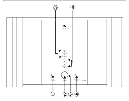
① The static bias model selecting button( select Class A/ Class AB/ AUTO mode by turns)
