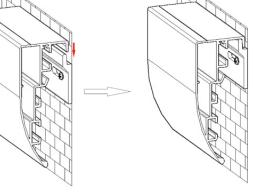
Then you simply hang the frame onto the two brackets and slide it into perfect position.
