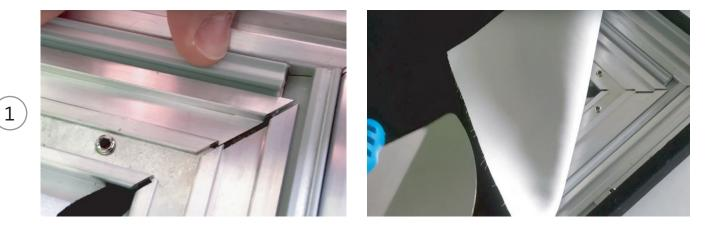
First, cut (use a regular cutting plier) the grip rails and insert them into the pre-fitted tracks. No glue is needed. Then place the fabric atop leaving the integrated, separate protective clothing underneath the frame and start tucking. **PS!** We recommend running the tucking tool through the rails first to open the slot as it is very tight from factory. This will make is far easier tucking the fabric afterwards.
