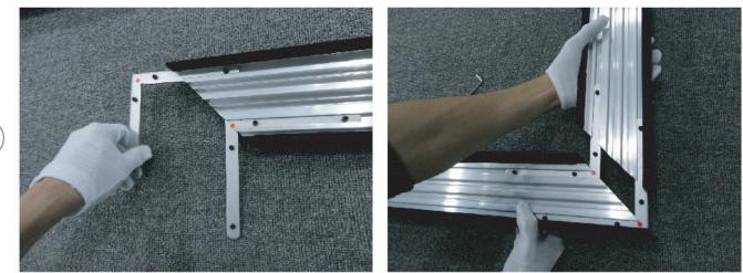
Then, attach the short sections and secure them by tightening the screws.
