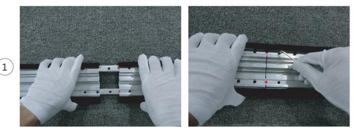
First, attach the long sections and secure them by tightening the screws.
