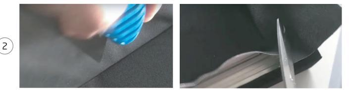
Start tucking in the fabric, long sides first, then the short sides. If needed, you can still easily pull out and re-tuck the fabric. When finished, cut of excessive fabric.
